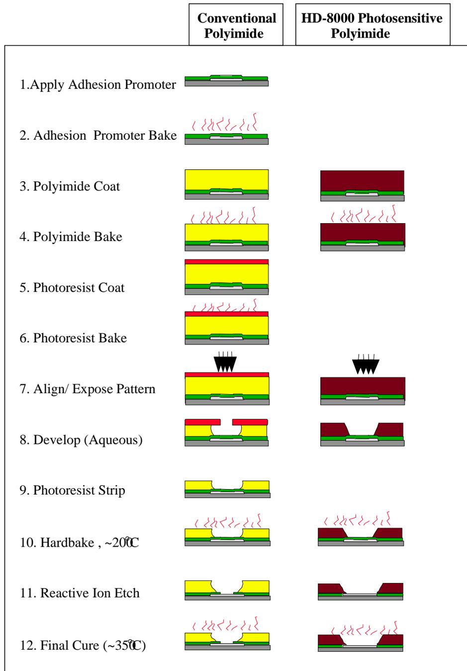
**Figure 1:** Comparison of conventional polyimide process and positive acting photosensitive polyimide process. The photosensitive polyimide process eliminates multiple steps and decreases cycle time.
