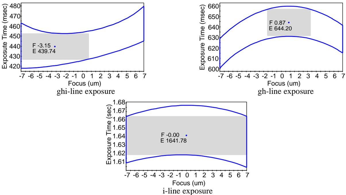
**Figure 5b:** Process window for 10µm spacewidth in 19µm thick HD-8000 polyimide exposed in ghi-line, gh-line and i-line. The process envelope shows ±10 percent CD control limits.
