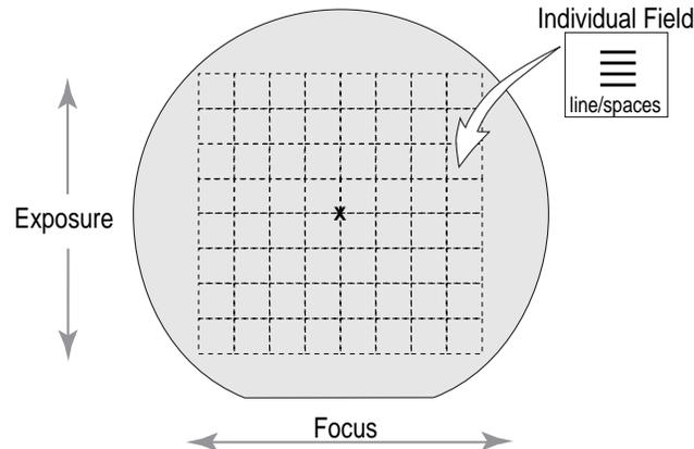
**Figure 3:** Wafer layout for the focus and exposure test matrix. An eight by eight field array was exposed with focus varying in the horizontal axis and exposure dose varying on the vertical axis.
