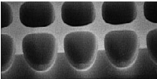
(a) 2.0 $\mu$ m vias on a 6  $\mu$ m pitch
