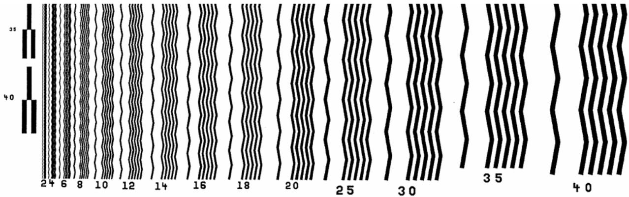
**Figure 2:** Partial view of the photomask layout showing vertical grouped and isolated lines from 2 to 40µm in size. The long SEM lines are placed in a zigzag pattern to increase mechanical integrity of the photoresist.
