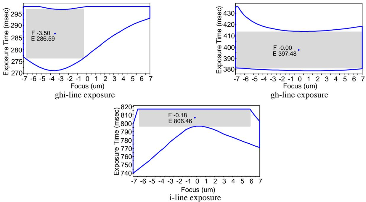
**Figure 6b:** Process window for 4 $\mu$ m spacewidth in 9.6 $\mu$ m thick HD-8000 polyimide exposed in ghi-line, gh-line and i-line. The process envelope shows  $\pm 10$  percent CD control limits.
