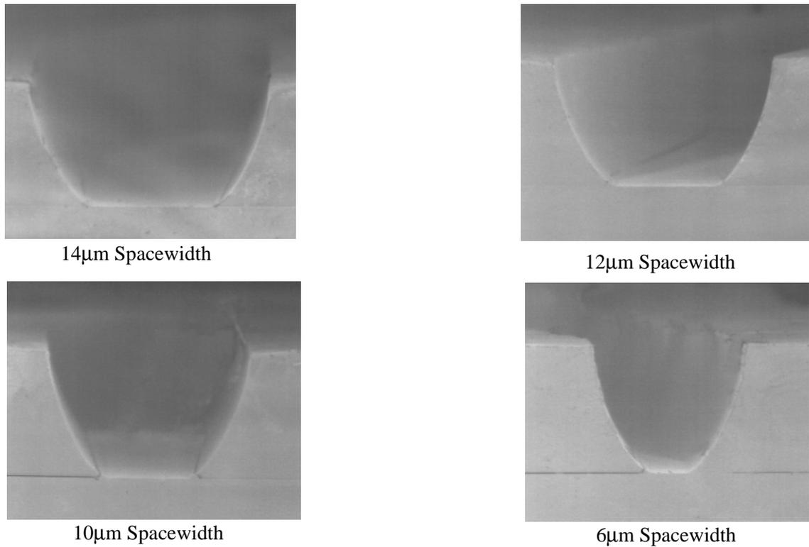
**Figure 5a:** Spacewidth linearity for 19µm thick HD-8000 polyimide exposed with ghi-line illumination. The exposure time is 440 msec (490 mJ/cm<sup>2</sup>) and the focus offset is -3µm.
