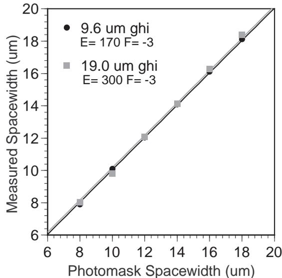
**Figure 4:** Mask linearity plot for 19.0µm and 9.6µm thick HD-8000 polyimide using a ghi-line stepper. The reticle bias was determined for each photoresist by regression analysis and is summarized in Table 5.
