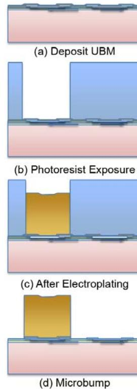
**Figure 3:** Process Flow showing (a) the deposited UBM (brown), (b) photoresist (blue) after development, (c) after Cu and solder electroplating (gold) and (d) the final bump after photoresist strip and UBM etching.
