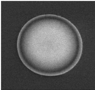
**Figure 13:** Top down SEM image of a  $3.5\ \mu\text{m}$  via at nominal conditions of  $1800\ \text{mJ}/\text{cm}^2$  and zero focus.
