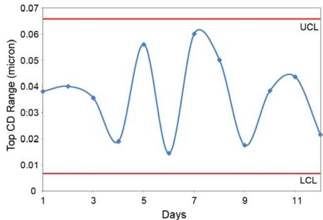
**Figure 17:** Range control chart for top CD showing stability of within wafer performance.
