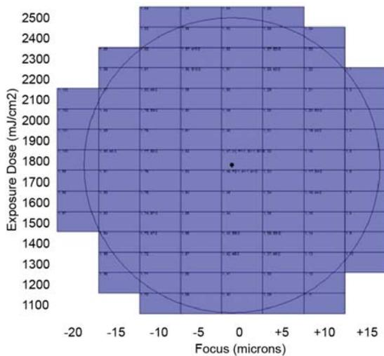
**Figure 4:** Wafer layout for the FEM. An eight by fifteen array was exposed with focus varying in the horizontal axis and exposure dose varying in the vertical axis.
