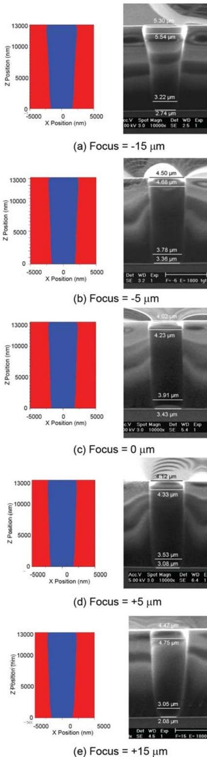
**Figure 9:** Comparison of simulated and experimental photoresist cross sections of 3.5  $\mu\text{m}$  vias through -15 to +15  $\mu\text{m}$  focus offsets. The photoresist thickness is 13.2  $\mu\text{m}$  and the exposure dose is 1800  $\text{mJ}/\text{cm}^2$ .
