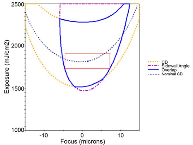
**Figure 10:** Modeled process window for 3.0  $\mu\text{m}$  via at 8  $\mu\text{m}$  pitch and photoresist thickness of 11.3  $\mu\text{m}$ . The DOF is 11.77  $\mu\text{m}$  and the nominal dose is 1825  $\text{mJ}/\text{cm}^2$ .
