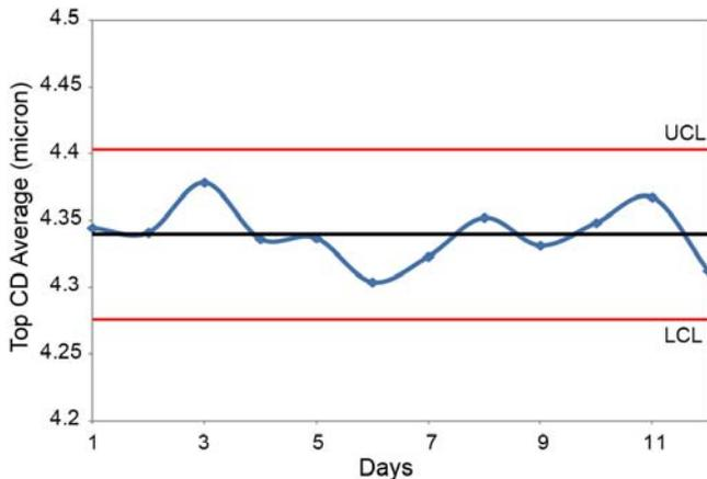
**Figure 16:** Average control chart for top CD showing the stability of the wafer to wafer performance.
