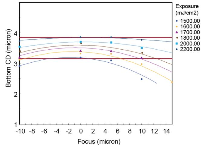
**Figure 5:** Bossung Plot for  $3.5 \mu\text{m}$  via hole with a pitch of  $10\mu\text{m}$  using bottom CD data from top down CD SEM.
