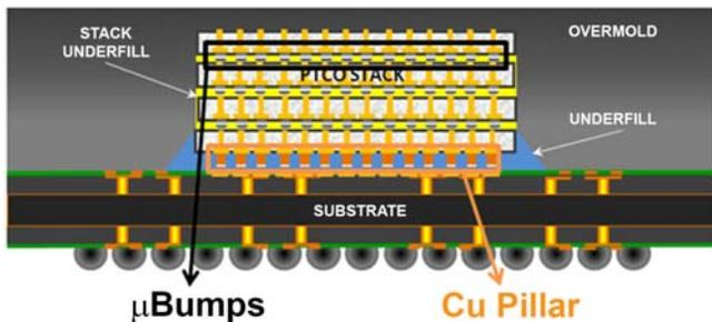
**Figure 2:** Drawings of a typical 3D stack showing the microbumps and Cu pillars.
