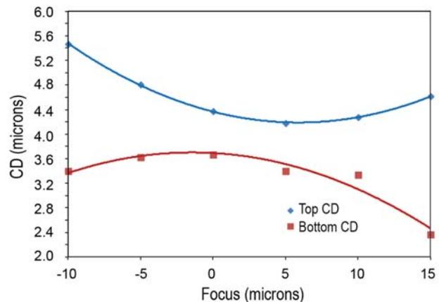
**Figure 15:** CD versus focus at  $1800\ \text{mJ}/\text{cm}^2$  for top CD (blue) and bottom CD (red) for  $3.5\ \mu\text{m}$  via with a pitch of  $10\ \mu\text{m}$  and a photoresist thickness of  $13.2\ \mu\text{m}$  as measured with top down CD SEM.
