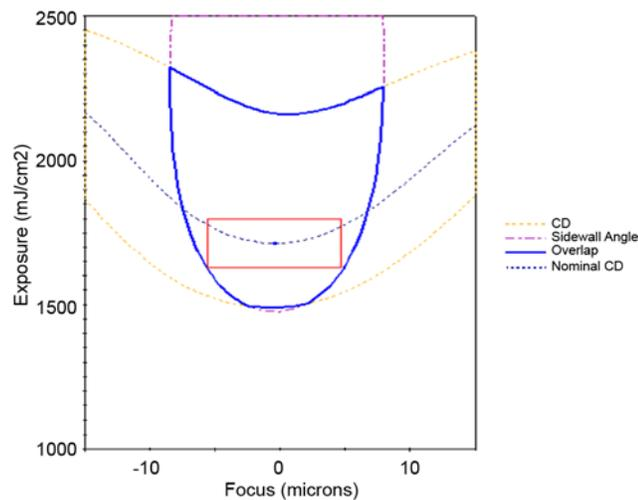
**Figure 7:** Experimental process window for 3.5 μm via using bottom CD data with a pitch of 10 μm and a photoresist thickness of 13.2 μm. The DOF is 10.0 μm with a nominal exposure dose of 1700 mJ/cm<sup>2</sup>. Sidewall angles were determined by cross sectional CD SEM.
