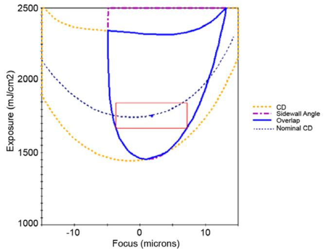
**Figure 8:** Modeled process window for 3.5 μm via at 10 μm pitch and resist thickness of 13.2 μm. The DOF is 10.86 μm with a nominal exposure dose of 1750 mJ/cm<sup>2</sup>.
