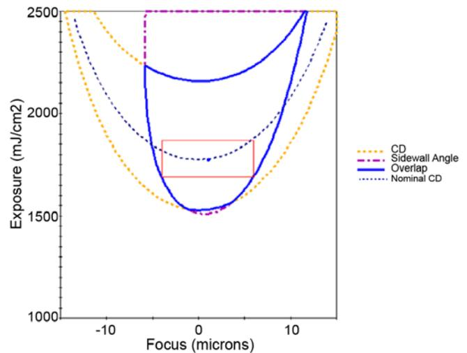
**Figure 11:** Modeled process window for 2.5  $\mu\text{m}$  via at 6  $\mu\text{m}$  pitch and photo resist thickness of 9.4  $\mu\text{m}$ . The DOF is 9.93  $\mu\text{m}$  and the nominal dose is 1775  $\text{mJ}/\text{cm}^2$ .
