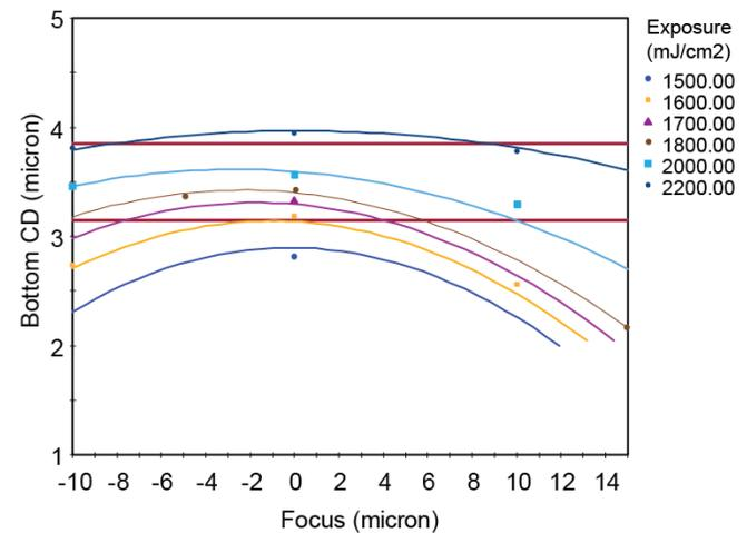
**Figure 6:** Bossung Plot for  $3.5 \mu\text{m}$  via hole with a pitch of  $10\mu\text{m}$  using bottom CD data from cross sectional CD SEM.
