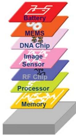
**Figure 1:** 3D stacking provides heterogeneous integration of different chip blocks to provide a complete a system on chip solution [2].
