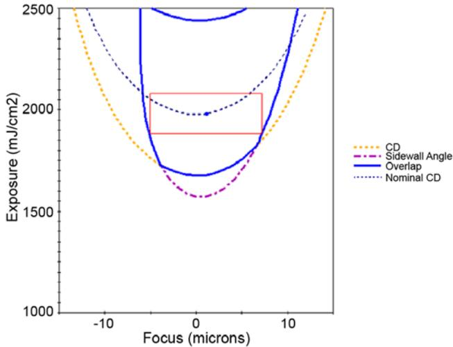
**Figure 12:** Modeled process window for  $2.5\ \mu\text{m}$  via at  $6\ \mu\text{m}$  pitch using a biased  $2.4\ \mu\text{m}$  feature on reticle. This increases the DOF from  $9.93$  to  $12.32\ \mu\text{m}$ . This nominal dose increases to  $1975\ \text{mJ}/\text{cm}^2$ .
