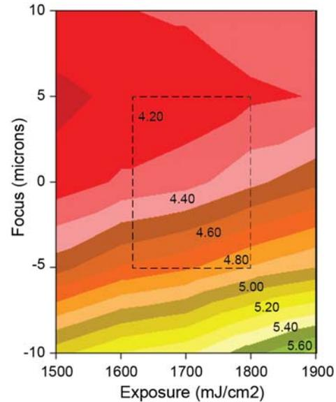
**Figure 14:** Contour plot of top CD data ( $\mu\text{m}$ ) as a function of Focus and exposure for  $3.5\ \mu\text{m}$  via with a pitch of  $10\ \mu\text{m}$  and a photoresist thickness of  $13.2\ \mu\text{m}$ .
